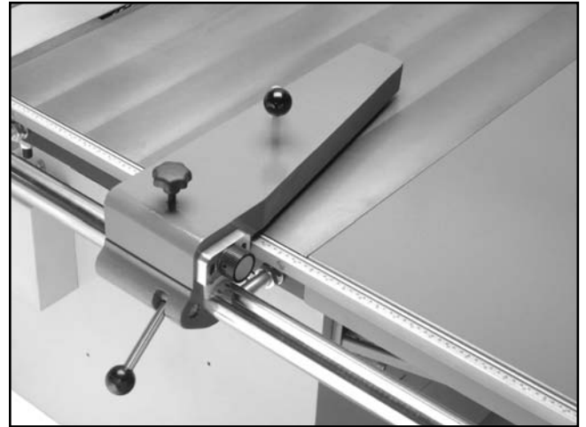
Figure 43. Installed clamp assembly.
